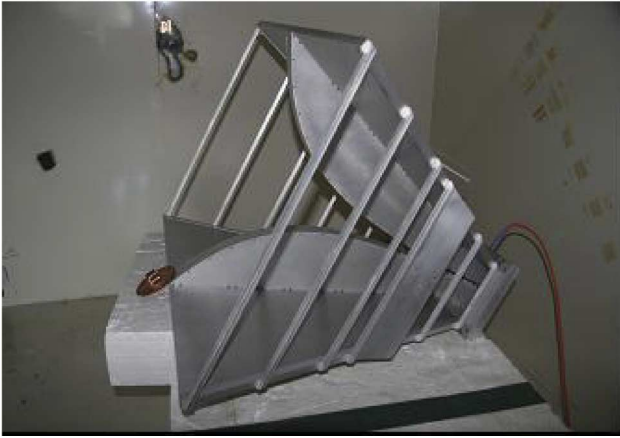
Fig. 3. Comparison of the 570-MHz small ground plane Z antenna and the dual-ridged reference horn in the NIST–Boulder reverberation chamber.
