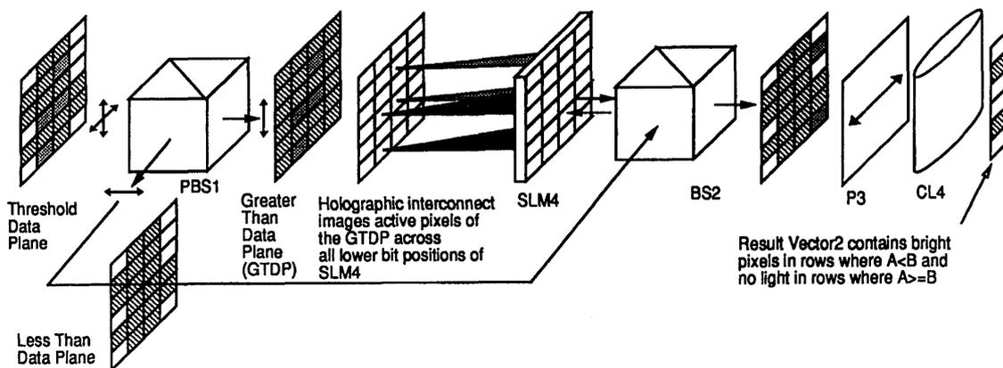
Fig. 2. Optical implementation of the single-iteration threshold unit.
