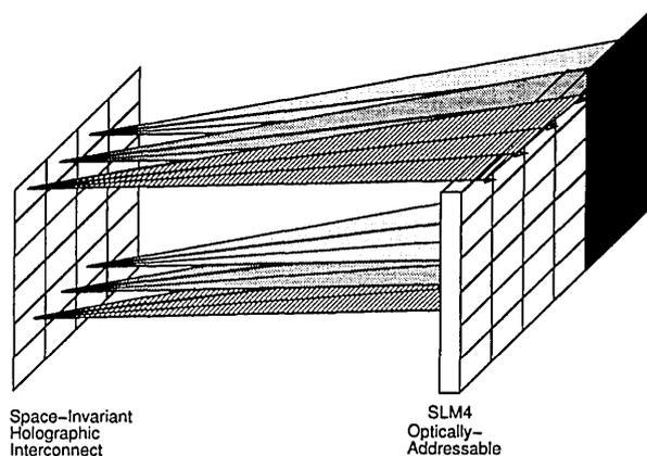
Fig. 3. Space-invariant hologram images each bit position of the incident data plane onto the corresponding lower bit positions of SLM4. Optics between the hologram and SLM4 remove unwanted diffraction orders and collimate the beams illuminating the SLM; these were omitted for clarity. The black wall attached to SLM4 serves as a baffle to block light beyond the SLM boundaries.
