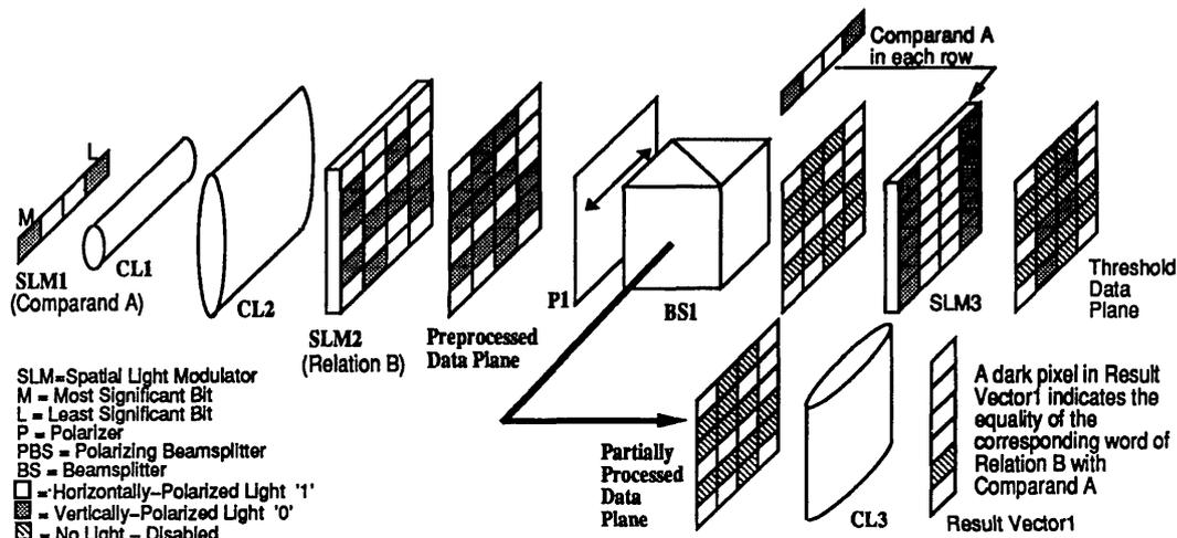
Fig. 1. Optical system for comparing an argument, Comparand A, with the attributes of Relation B.
