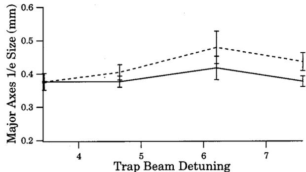
FIG. 7. The  $1/e$  trap radius  $a$  along the  $\hat{z}$  axis as a function of trap laser beam detuning in units of the natural linewidth ( $\gamma=5.9$  MHz). The solid line shows the fit when the pulse area is held constant; the dashed line shows the fit when the pulse area is varied.
