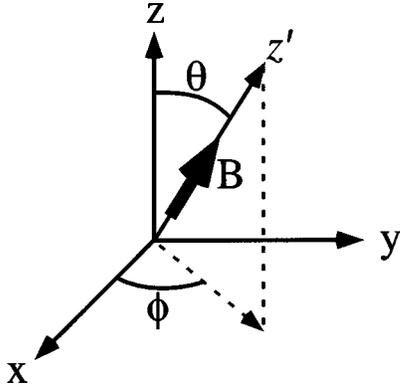
FIG. 9. Orientation of the quantization axis  $\hat{z}'$ . The primed axes are the atom frame coordinates, determined by the components of the magnetic field; the unprimed axes are the lab frame coordinates. The  $\hat{z}$  axis is the propagation direction of the Raman fields.
