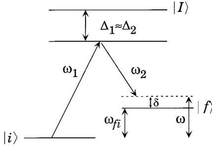
FIG. 1. Energy-level diagram for the Raman transition.
