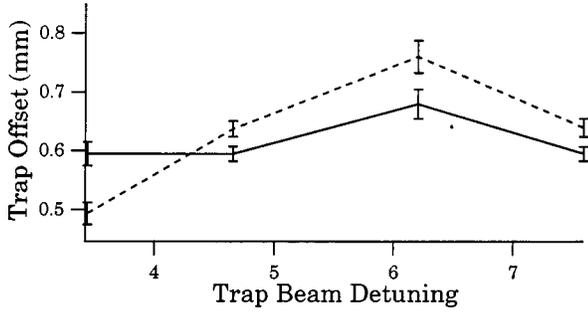
FIG. 8. The offset of the trap along the  $\hat{z}$  axis as a function of trap laser beam detuning in units of the natural linewidth ( $\gamma=5.9$  MHz). The solid line shows the fit when the pulse area is held constant; the dashed line shows the fit when the pulse area is varied. The offset perpendicular to the  $\hat{z}$  axis is found to be negligible. Note that the offset is measured with respect to the magnetic-field zero point.
