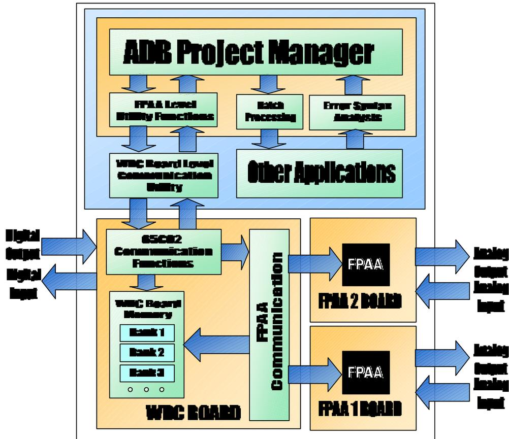
Figure 1. Block diagram of analog-digital development system.
