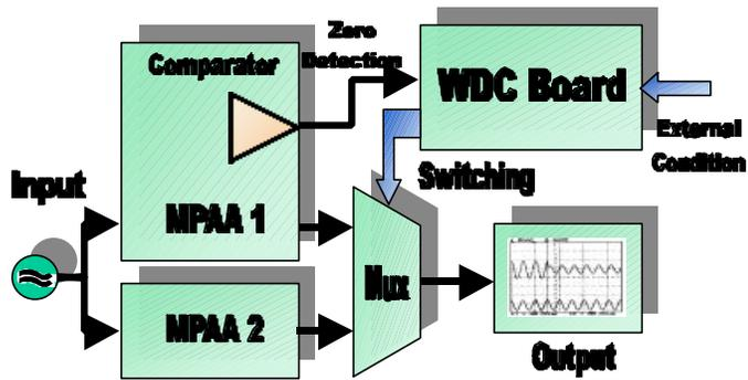
Fig. 3. Schematic of implementation of adaptive filter with use of 2 FPAA's and an analog multiplexer (*MUX*).
