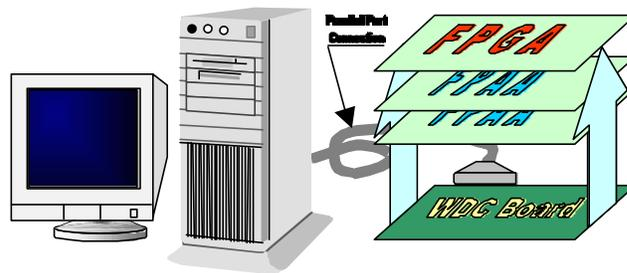
Figure 4. Physical arrangement of FPAA's, FPGA, WDC development board, PC , and monitor for experimental implementation of adaptive filtering.
