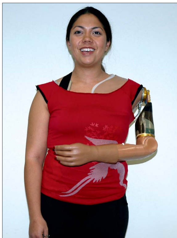
Figure 10: Experimental prosthesis consisting of a motorised elbow, wrist, and hand, with passive shoulder components
