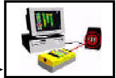
download program to the robot RCX using IR (infrared transmitter)
