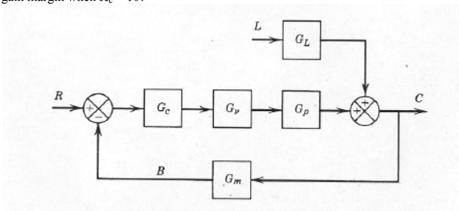
3) Problem 16.12 from first edition - The block diagram of a conventional feedback control system contains the following transfer functions:
