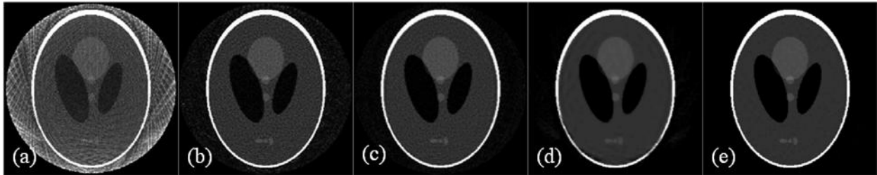
Figure 5: Phantom images reconstructed from 32 radial views using (a) NUFFT+SOS (b) CG-SENSE (c) CG-SENSE with Tikhonov regularization (d) CS + SOS (e) PICS.
