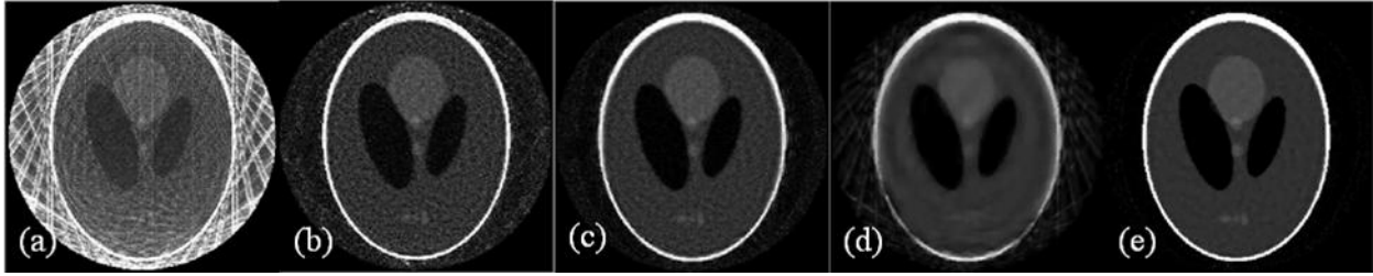
Figure 4: Phantom images reconstructed from 16 radial views using (a) NUFFT+SOS (b) CG-SENSE (c) CG-SENSE with Tikhonov regularization (d) CS + SOS (e) PICS.
